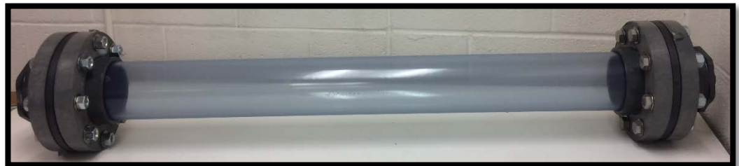
Assembled clinoptilolite column
