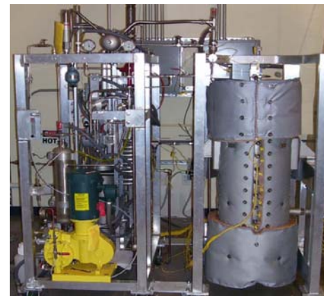
10 kg/day Hydrogen Pilot Plant
